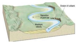
Fig. 2. Erosion deposition in meandering stream
