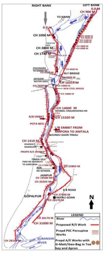
Fig. 4. Location of anti-erosion and river training work
