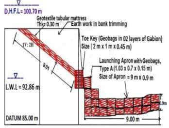
Fig. 6. Typical cross section of bank revetment and apron
